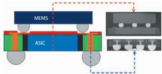
Figure 6. 3D eWLB for MEMS/Sensor Devices[8].
