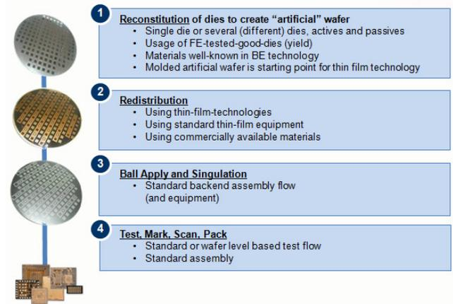
**Figure 2. Process flow of eWLB assembly**
