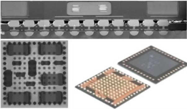
Figure 5. Photographs of 3D SiP eWLB-PoP with discrettes on interposer or top package of discrettes.
