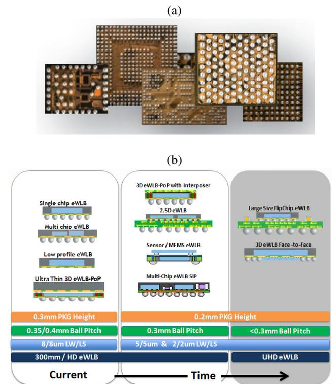
Figure 1. (a) eWLB packages and (b) evolution of eWLB technology from 2D to 2.5D/3D packaging solution
