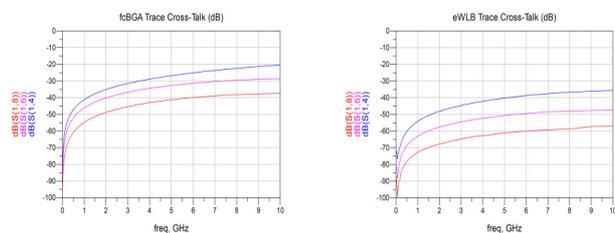
**Figure 3. The cross-talk with frequency of signal routing of (a) flipchip and (b) eWLB.**
